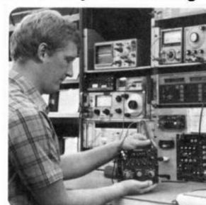
SERVICE IS OUR BUSINESS — Richard Rysstrom, electronics technician, checks the performance of a Collins ANARC-182 radio set.
